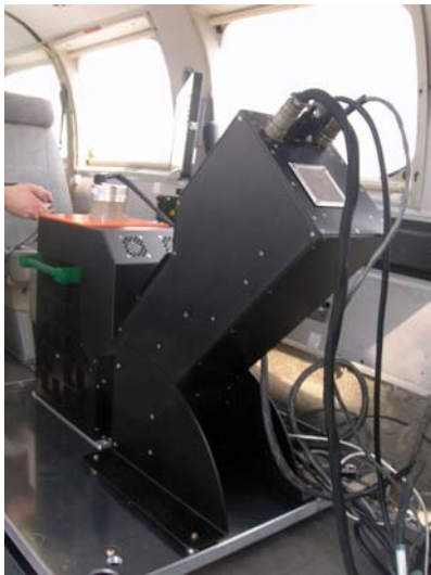
Figure 12: MASI hyperspectral imager sensor head mounted in a fixed-wing aircraft
