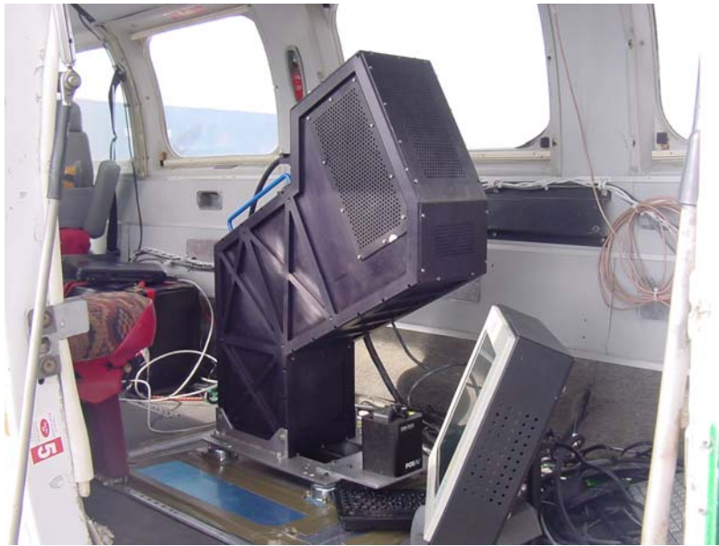
Figure 1: TASI hyperspectral imager sensor head mounted in a fixed-wing aircraft
